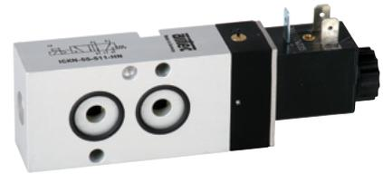
Electrically operated spool valve. The manual override is detent and is operated by screw driver. The location pin, screws and seals are included.
